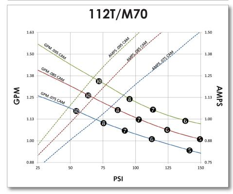
Data recorded pumping water at room temperature and 115V AC power. Actual performance will vary with voltage, application, and mfg tolerances. Copyright Pumptec, Inc. 2014
