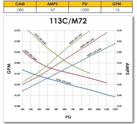
Data recorded pumping water at room temperature and 230VAC 50Hz power. Actual performance will vary with voltage, application, and mfg tolerances. Copyright Pumptec. Inc. 2014
